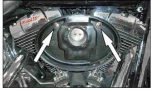
5. Remove the two crankcase bolts as shown
