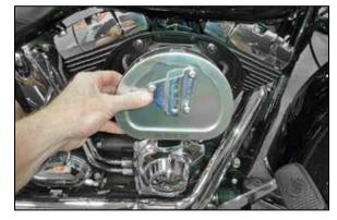
Remove the air filter with breather hoses as shown.
