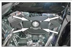
11. Install the provided gasket between the back plate and air filter base using provided hardware. Slightly tighten at this time. Using the air filter cover clock the filter base in position then finish tightening filter base plate.
