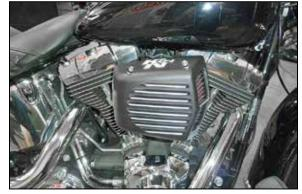
12. Install air filter and air filter cover with provided bolts.
