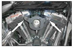
9. Using the two provided crankcase breather bolts install the back plate onto the vehicle as shown. Do not tighten the breather bolts at this time.
