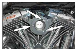
10. Install the provided gasket between the throttle body and back plate use the provided hardware to secure the back plate to the throttle housing. Tighten the crankcase breather bolts.
